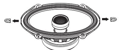
If a clearance is found between the vehicle side panel and the speaker unit, glue the cushion ⑨ supplied on surface of the speaker gasket.
